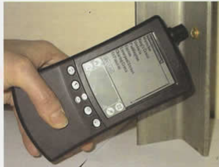
BELOW: Interrogating a tag with a PDA
